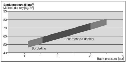
1) The processing behaviour was determined on moulded parts measuring 300 x 200 x 60 mm, which were produced under standard conditions at a vapour deposition pressure of 3.2 to 3.6 bar. The specifications refer to medium bulk densities
